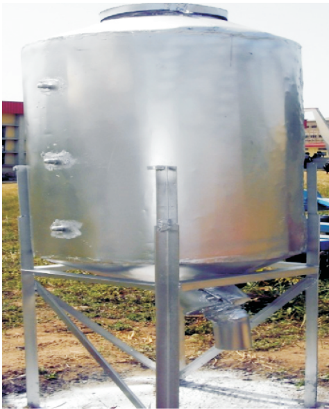
Plate VI: The Double-Walled Metallic Silo
