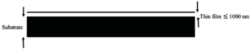
Fig. 5: Thin solid film on a substrate
