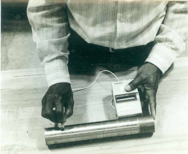
Plate 4: Measuring Surface Roughness of Machined Pieces with Surf-Indicator
