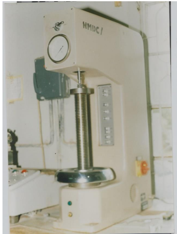
Plate 8: Karl Frank GMBH Rockwell Hardness Testing Machine
