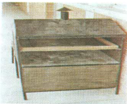
Plate 3: Natural airflow cabinet dryer used in drying differently salted O. niloticus Designed by Z. D. Osunde, (2002).
