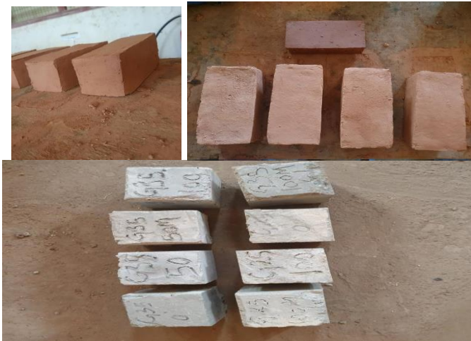
Plate 16 Cement concretes and clay bricks processed with zymocrete. The samples were 3x stronger than conventional concretes and clay bricks
