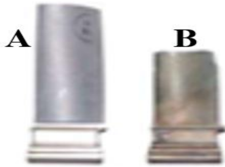
Figure 15: Gas Turbine Blades: (A) – a new turbine blade, (B) – the in-service damaged one (Orah et. al. , 2019)
