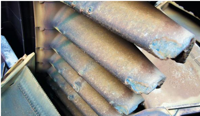
Figure 18: Degraded Turbine Blade Tips. (Nasir, et. al. , 2016)
