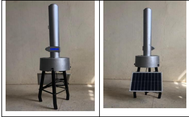
Figure 21: The IoT greenhouse gases data logger (Ndaliman, et al., 2024)
