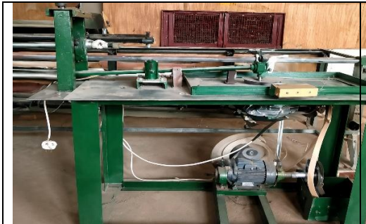
Figure 24: The Pin-On-Disc Wear Testing Machine
