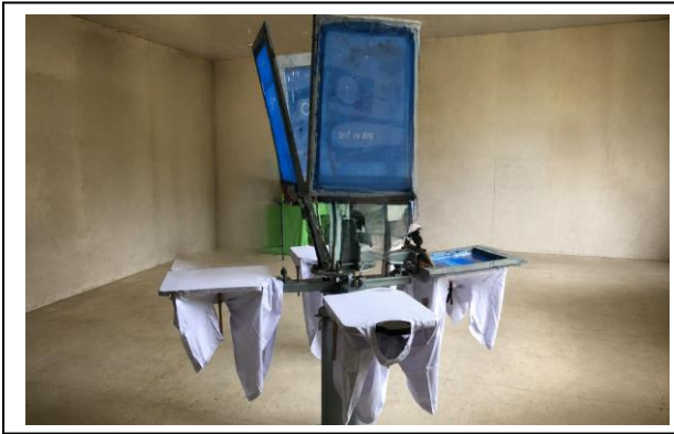
Figure 22: Four Stations Four-Colour Screen-Printing Machine (Ndaliman, 2022)
