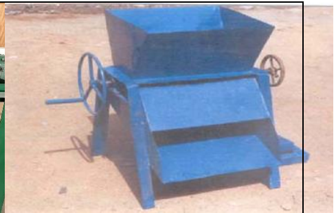
Figure 25: A Dual - Operational Cassava Grating Machine
