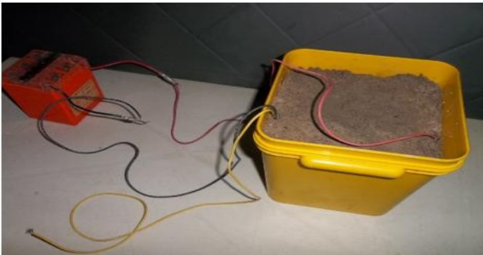
Figure 10: Impressed current cathodic protection setup
